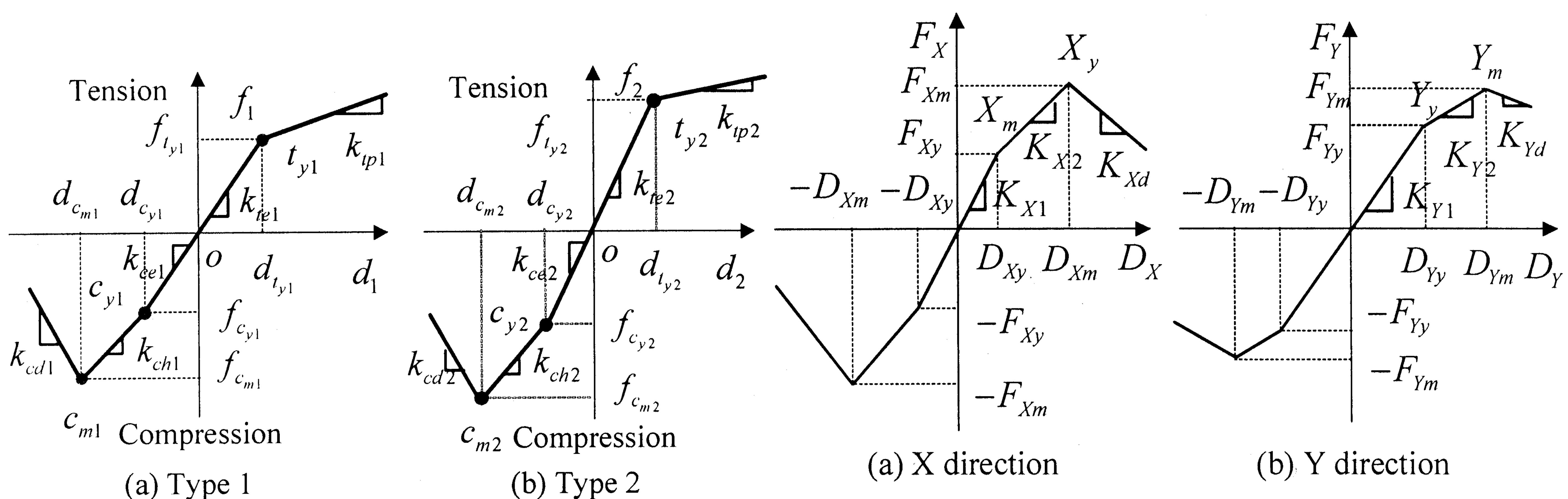
Figure 2 Two types of skeleton curves of spring
