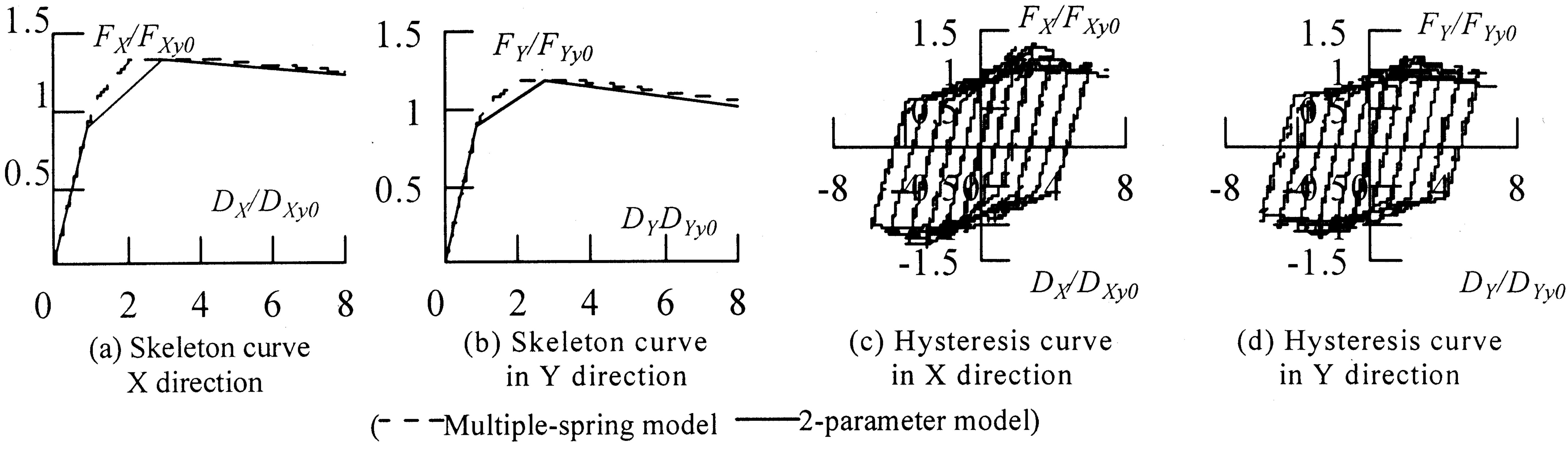
Figure 4 Comparison between multiple-spring model and 2-parameter model
