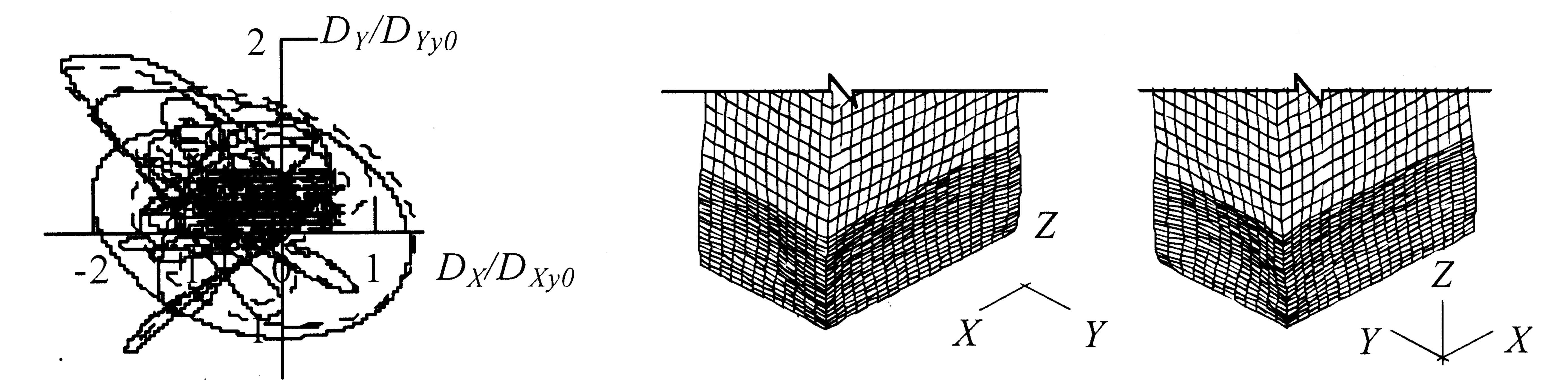
Figure 5 Trajectory of response sway displacement on X-Y plane under JMA wave
