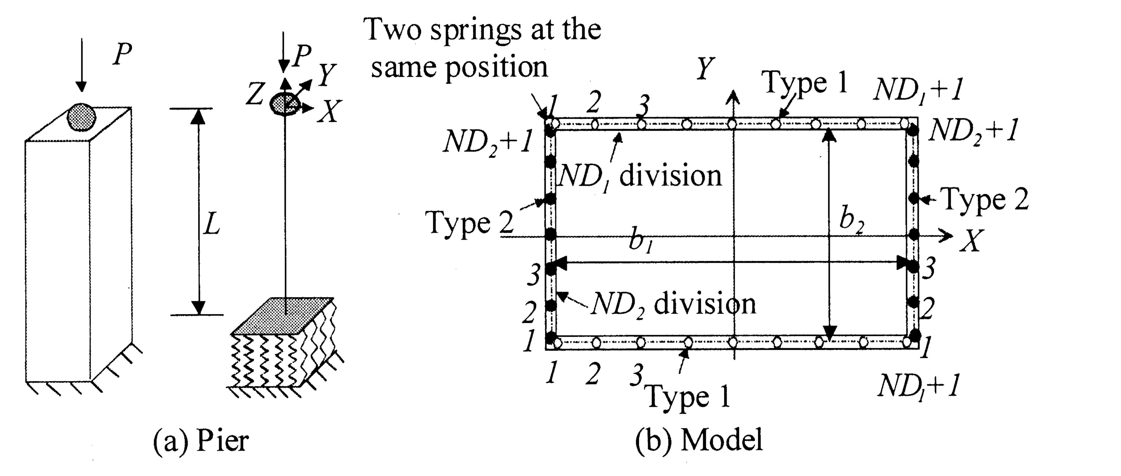
Figure 1 Multiple Spring Model
