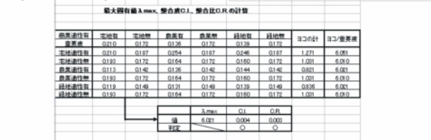
Figure 10 Example of spread sheet design for inputting the pairwise comparison values and calculating the degree of importance.
