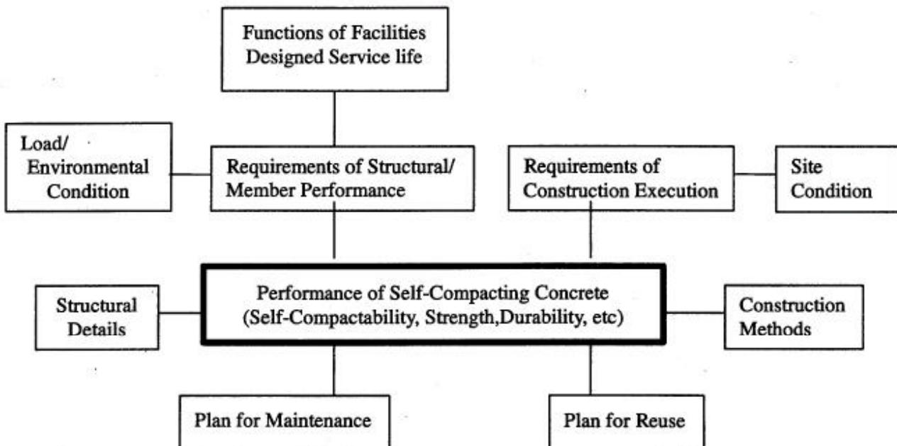
Fig. 2.1 Relations between Performance of Self-Compacting Concrete and Others
