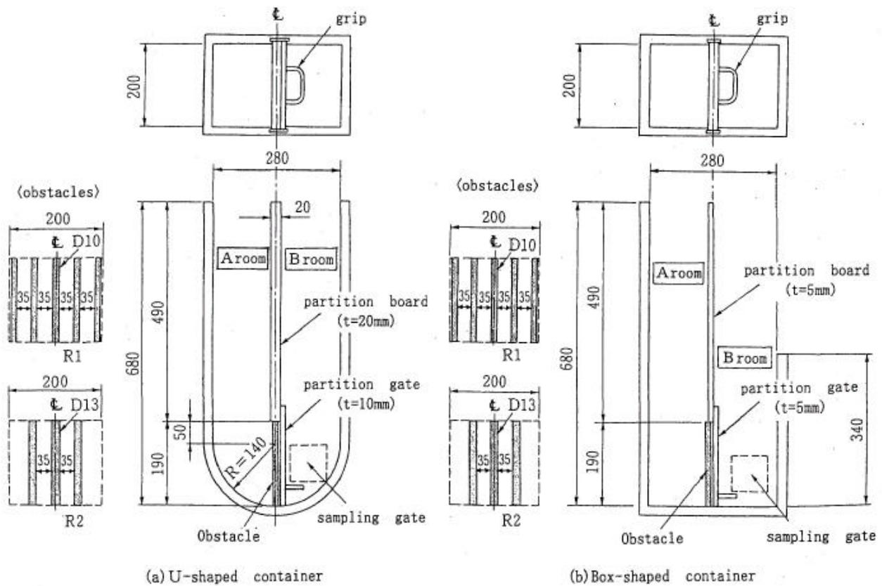
Fig.5. 1 Shapes and Dimensions of Apparatus for Self-Compactability Test
