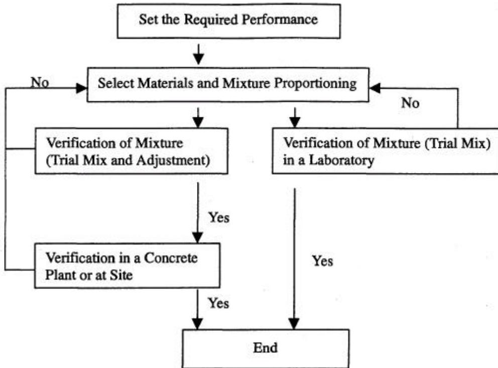
Fig.4.1 Flow Chart of Mixture Proportioning
