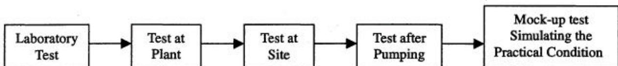
Fig.5.2 Timing of test for verification of Self-compactability
