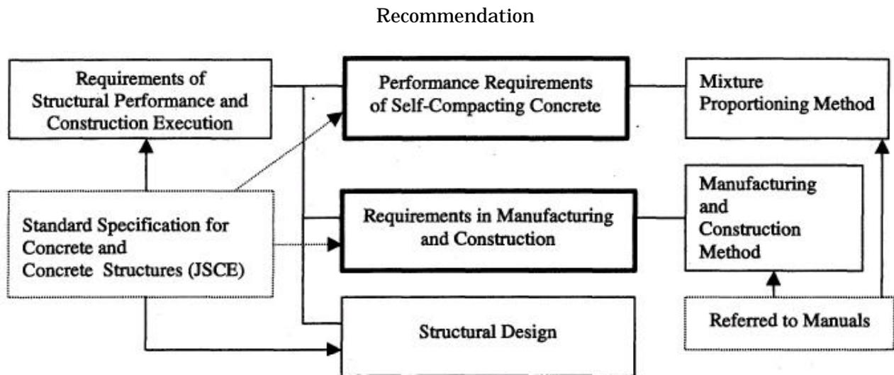
Fig. 1. 1 Scope of Recommendation for Self-Compacting Concrete
