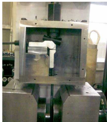
Photo 3. Strength test for corner support material
