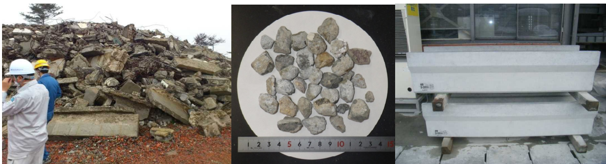
Figure 4. Precast concrete with recycled aggregate made from concrete rubble (Kitatsuji et al.)
