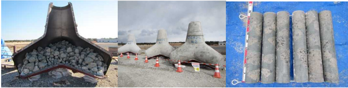
Figure 5. Wave-dissipating blocks made using the pre-packed method with seawater and concrete rubble of large particle size (Katano et al., Report by Obayashi Corporation Technical Research Institute)
