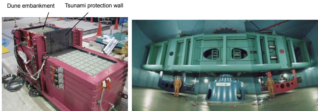
Figure 4. Centrifugal model experiment (left: test specimen; right: centrifugal loading device)
