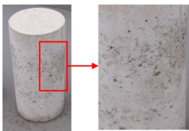
Photograph 2 Example of sanding phenomenon Surface roughness and peeling
