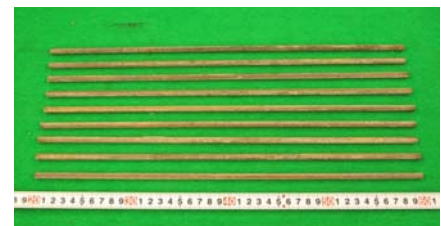
Photo 4 Post-tensioning wires (C2 wires)
