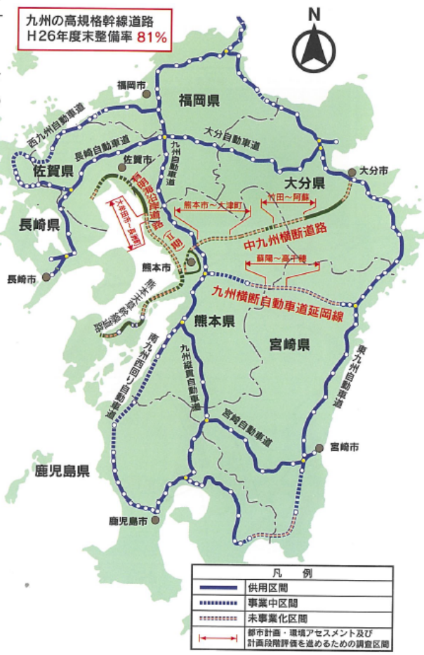
Figure 1 Arterial roads and regional arterial roads in Kyushu including Kumamoto Prefecture (extracted from “Rivers and Roads in Kumamoto 2015”)
