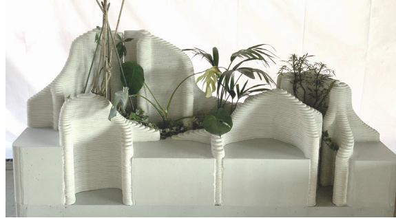
Photo 2: Eco-friendly bench fabricated by 3DCP with carbon-negative substitute
