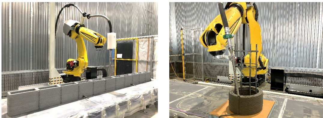
Photo 5: 3DCP technique with a robotic arm on a slider
