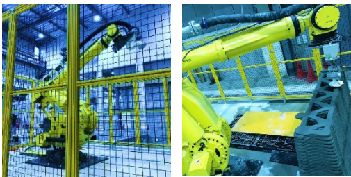
Fig.3 Robot arm-type 3D printer and printing
