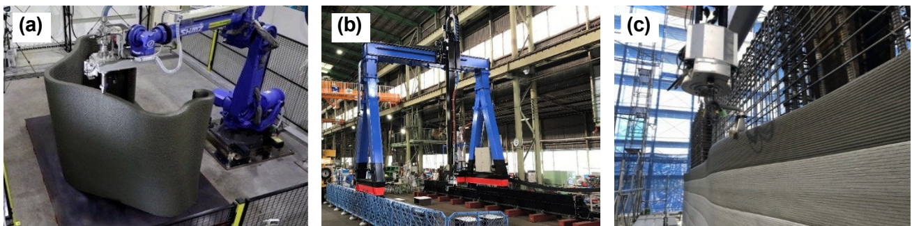
Fig. 1 Printing system using (a) a robotic arm and (b, c) a gantry system.
