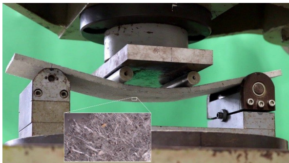
Fig. 2 Deflection hardening behavior of LACTM (inset: magnified image of crack plane).
