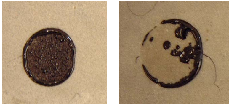
Figure 8.13 – Type of failure from the PATTI-test (left: cohesive failure, right: adhesive failure)
