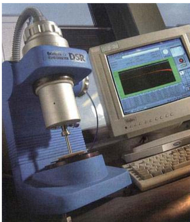
Figure 2.7 – Dynamic Shear Rheometer (reproduced with kind permission from The Shell Bitumen Handbook [2.31])
