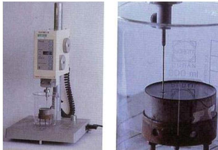
Figure 2.16 – Penetration test (reproduced with kind permission from The Shell Bitumen Handbook [2.31])
