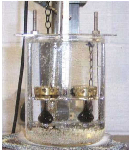
Figure 2.19 – Softening point test (reproduced with kind permission from The Shell Bitumen Handbook [2.41])
