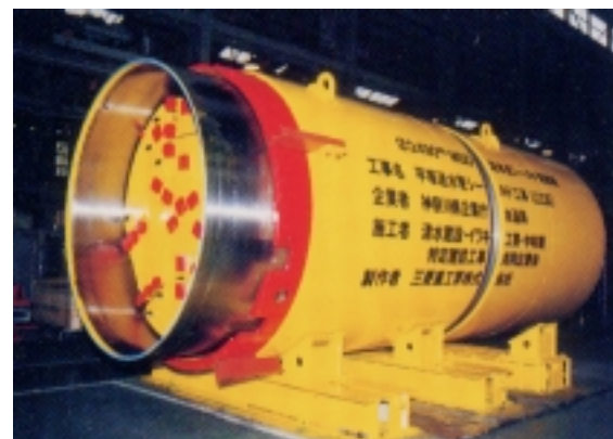
Shield Machine for MSD Method (Penetrating ring is extended for coupling)
